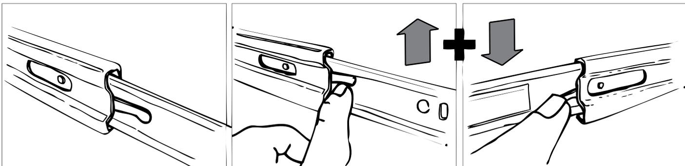
Fully extend drawer and locate plastic lever on drawer slide.
