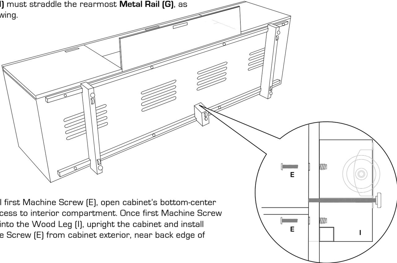
**NOTE:** To install first Machine Screw (E), open cabinet's bottom-center door to gain access to interior compartment. Once first Machine Screw (E) is threaded into the Wood Leg (I), upright the cabinet and install second Machine Screw (E) from cabinet exterior, near back edge of cabinet.
