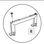
Carefully lay (C) Cabinet on its back. Using (B1) Hex Wrench, attach the base assembly to the bottom of the (C) Cabinet with (D) Screws and (G) Screws.
