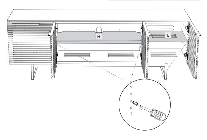
Levelers are integrated into each leg assembly and are accessed at the bottom of each cabinet leg using the (B2) Open Mouth Wrench. If your floor is uneven, you may extend one or more levelers to attain a level, stable cabinet placement. Turning the leveler clockwise will extend the leveler; turning it counter-clockwise will retract it.
