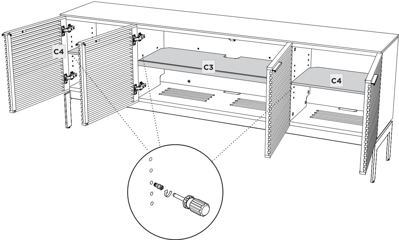
Levelers are integrated into each leg assembly and are accessed at the bottom of each cabinet leg. If your floor is uneven, you may extend one or more levelers to attain a level, stable cabinet placement. Turning the leveler clockwise will extend the leveler; turning it counter-clockwise will retract it.
