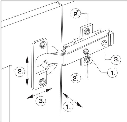
Use a Phillips screwdriver to adjust Mirage's door hinges:
