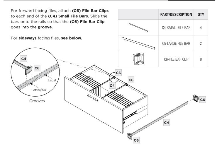
For letter files facing sideways, attach (C6) File Bar Clip to both ends of (C5) Large File Bar as shown. Place the file bar assembly in the notches located on the left and right drawer side panels. For side facing legal files, skip this step altogether and hang file folders directly on front and back rails.
