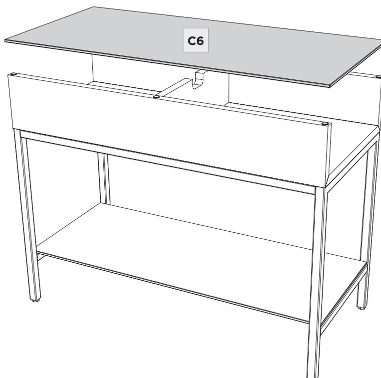
Make sure the table is level. Adjust one or more of the levelers using **(T2) Leveler Wrench** to attain a level stance.
